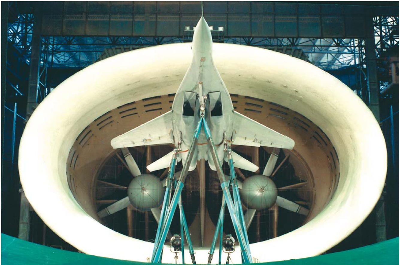
Mig 29 T-101 mock-up in course of aerodynamic tests in the wind tunnel of TsAGI. (Credit TsAGI)
