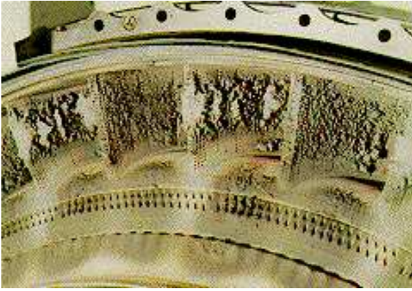
Figure 2. Part of an B-747 engine after flying through an ash plume, June 1982. [Source: http://www.geo.mtu.edu/departments/classes/ge404/gcmayber/engine.html ]
